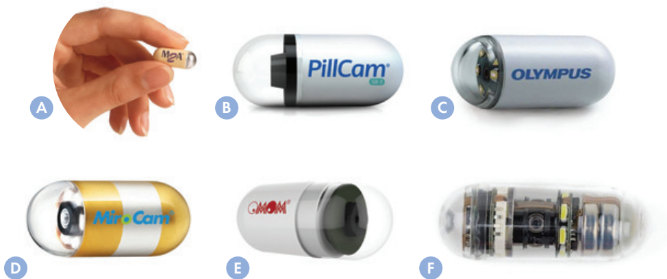
Figure 3 Commercially available SBCE (the first approved and the latest versions). A. M2A® (Given Imaging Limited, Yoqneam, Israel); B. PillCam® SB3 (Medtronic, Yoqneam, Israel). C. EndoCapsule® 10 (Olympus, Tokyo, Japan); D. MiroCam® MC1600 (Intromedic, Seoul, South Korea); E. OMOM® HD (Jlinshan Science and Technology Group, Chongqing, China); F. CapsoCam® Plus (CapsoVision, Cupertino, California, USA). Images extracted from Civi G, et al. (2016) and Moglia A, et al. (2007).
